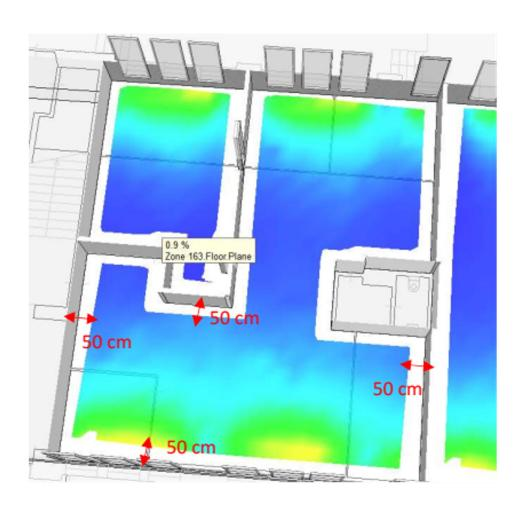
The uniformity ratio calculation, minimum point daylight factor and minimum daylight illuminance can exclude areas within 0.5m of walls. Areas within 0.5m are not regarded as part of the working plane for this purpose, although they are included in the average daylight factor and average daylight illuminance calculations.
